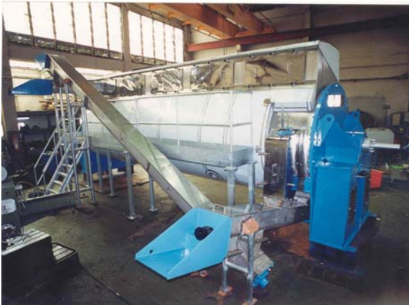
ASTW 160 sqm stainless steel blood dryer with recycling screw conveyors. Capacity up to 50 tons of raw blood per 24 hrs.
